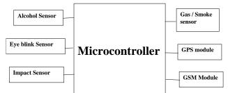
Figure 2 Real time driver monitoring
